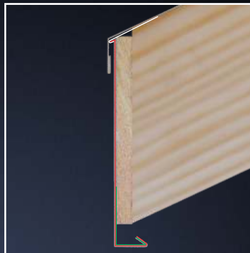
Cross-section after the installation of the flush-mounted strip.
