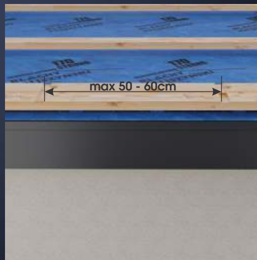
The remaining hooks are fastened at a maximum distance of 50-60 cm from each other.
