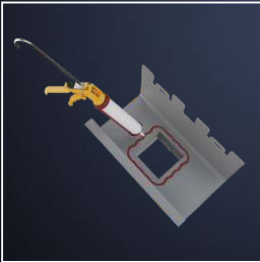
Application of binder to seal the connection between the gutter outlet and the outlet.
