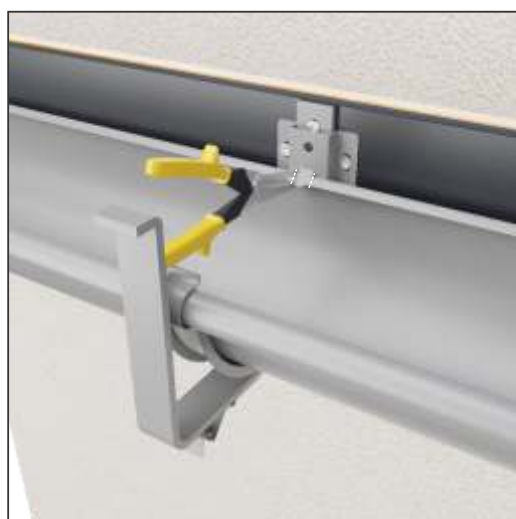
We create a fixed point of the expansion joint by cutting the rear stiffener on both sides of the central-most hook using left and right scissors. The fixed point of the middle hook shortens the expansion joint by half.
