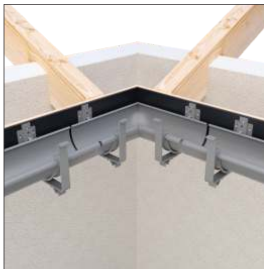
Gutters and corner mounted on hooks with a 5-10 mm expansion joint.
