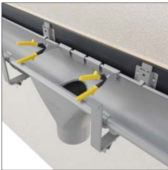
Incision of the rear stiffening of the gutter with left/right cutters - creating fixed points of the outlet that prevent its movement.
