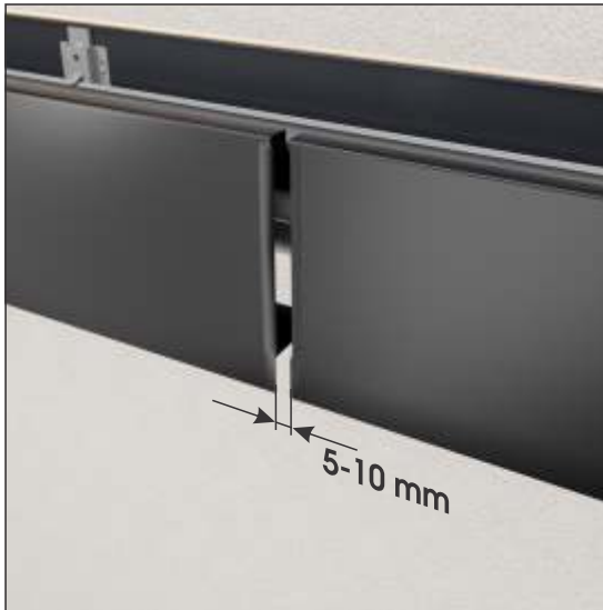
The cover plug installed with a 5-10 mm expansion joint. The joint with the gutter end should not be located in the location of a gutter joint.
