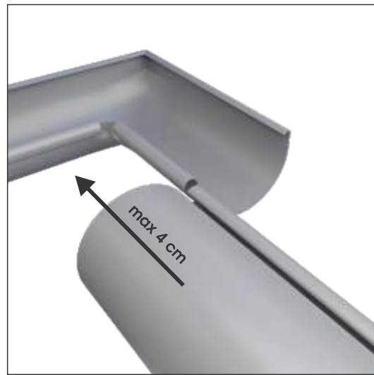
Placing the gutter into the corner. When joining gutters with corners by an overlap, an overlap of max. 4 cm is recommended.
