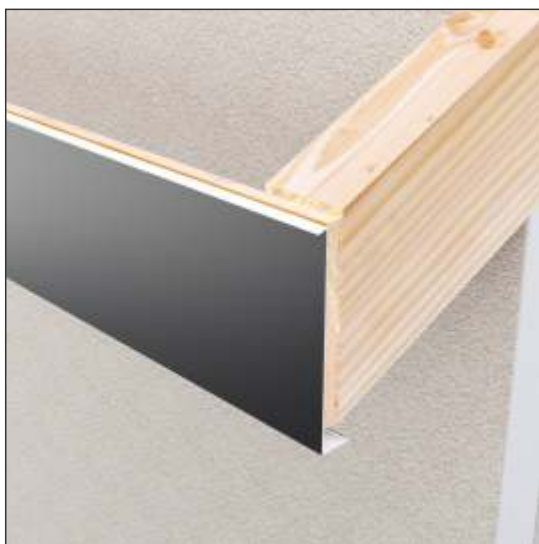
Attaching the cover to the starter strip. The lower bend enables the mounting of the soffit lining on the roof flashings - see the installation of the soffit lining on page 20.
