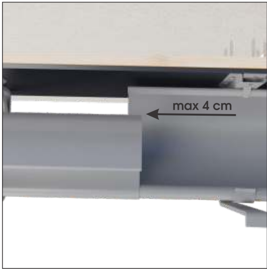
The gutters joined using an overlap. When joining gutters by an overlap, an overlap of max. 4 cm is recommended.
