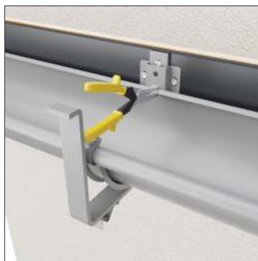
We create a fixed point of the expansion joint by cutting the rear stiffener on both sides of the central-most hook using left and right scissors. The fixed point of the middle hook shortens the expansion joint by half.
