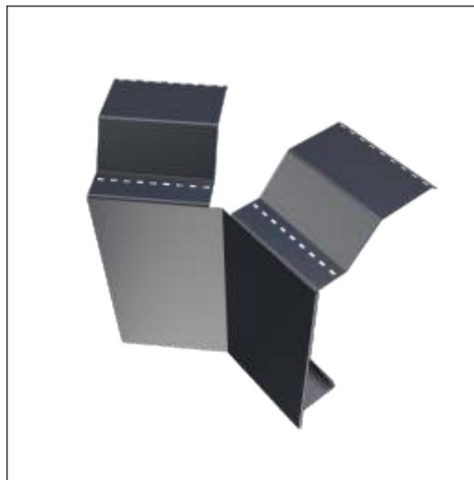
Deflected plug cover of a corner.
