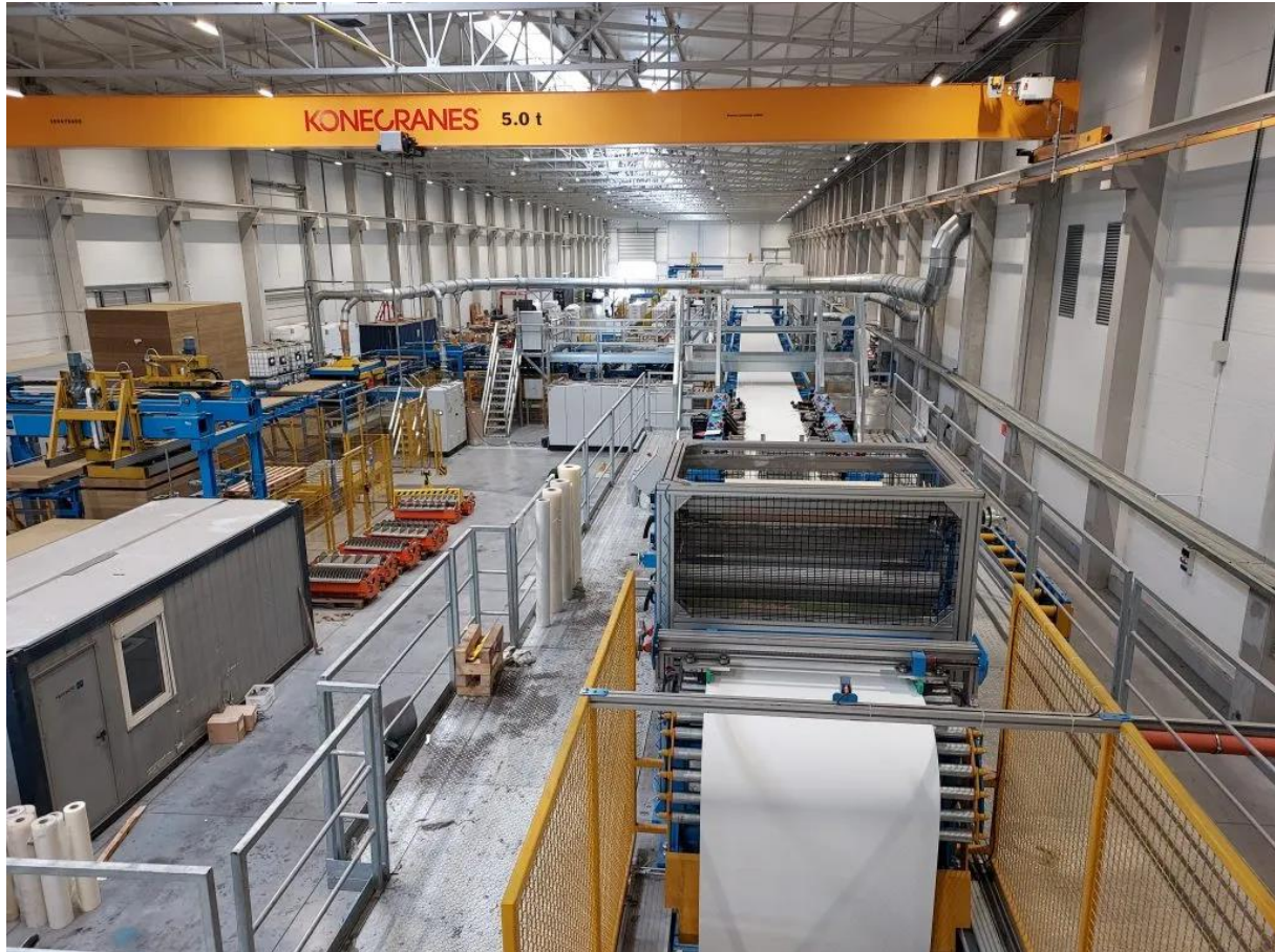
Figure 3.3: Technological line for the production of sandwich panels
