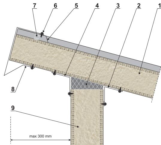
Roof panel PWD-PIR may be placed outside of the building wall contour maximum 300 mm.
