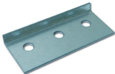
Strain Distributor is a necessary element during assembly of sandwich panels with hidden joint PIRTECH PLUS. Its exclusion decreases lifting capacity about 30%.
