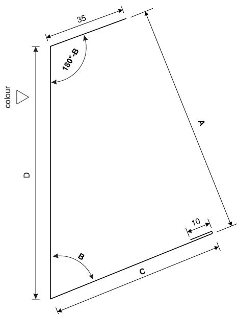
Flashing produced from sheet of thickness 1,00 mm
