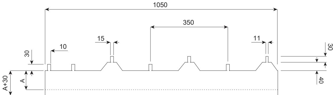
The „front cover” masking flashing is intended for the PWD-PIR roof sandwich panel and is fixed to the face of the panel. The A dimension depends on the board thickness. The dashed lines mark the places where the flashing should be bent at an angle of 90°.
