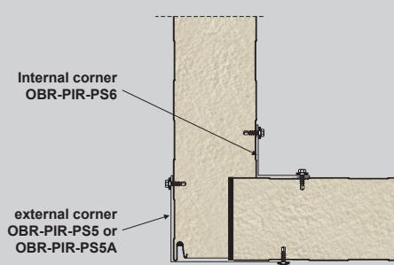
Indentation of panels allows for application of external corner flashing in one width no matter what kind of thickness will be used.
