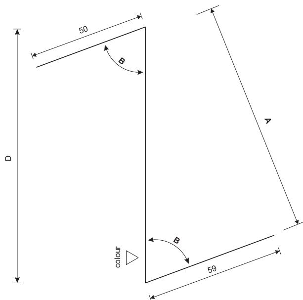
**Flashing produced from sheet of thickness 1,00 mm**
