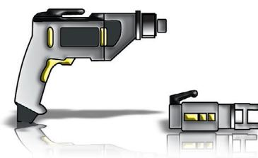
We recommend usage of specialized power tools – screwdrivers with a special head for proper fastening and limitation of fastening depth. The pressure of the connector should be adjusted in such a way not to deform the washers - as shown.
